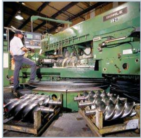
CycloBlower rotors are precision ground using state of the art milling technology.
